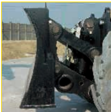
■ PARALLELOGRAM BLADE with two vertical cylinders
