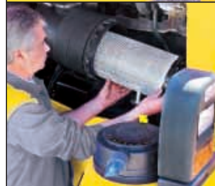
■ Side panel opening enables easy access to main engine components and facilitates filtre replacement
