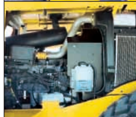
■ Side panel opening enables easy access to main engine components and facilitates filtre replacement
